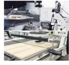
The P-System connectors Clamex, Tenso and Divario can be cut which enables corner, dividing panel and surface joints.
